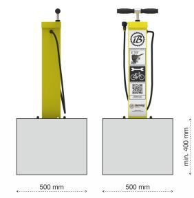
The **IBOMBO PRS–sv1** public bicycle pump is designed for use in public spaces. The advantage of this model is its small size, which allows it to be installed almost anywhere. In this model, it is not possible to hang the bike on the rack. The construction of the housing is made of a galvanized/stainless steel profile - powder coated or plastic coated. The device is fixed to the ground with anchors. The sheet metal elements of the device are connected with anti-theft screws.
